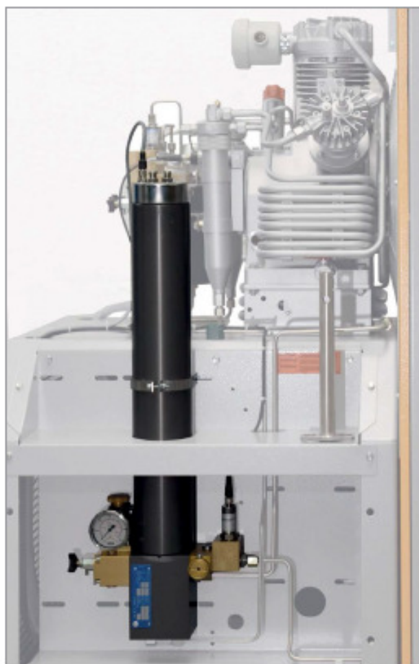
The P42 purification system with integrated separator
